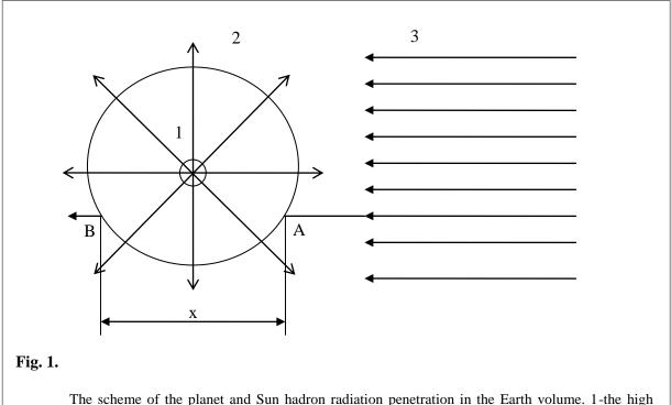
The scheme of the planet and Sun hadron radiation penetration in the Earth volume. I-the high temperature planet core; 2,3 - the hadron radiation of the planet and solar origin, correspondingly. A, B are the points of the day and night measurements, correspondingly; X is the planet chord length.
